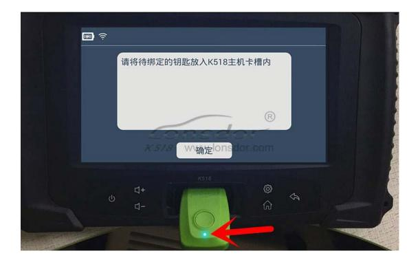
2. System will read backup data of vehicle to generate emulator key and prompt to choose corresponding key type(refer to back of the emulator).
